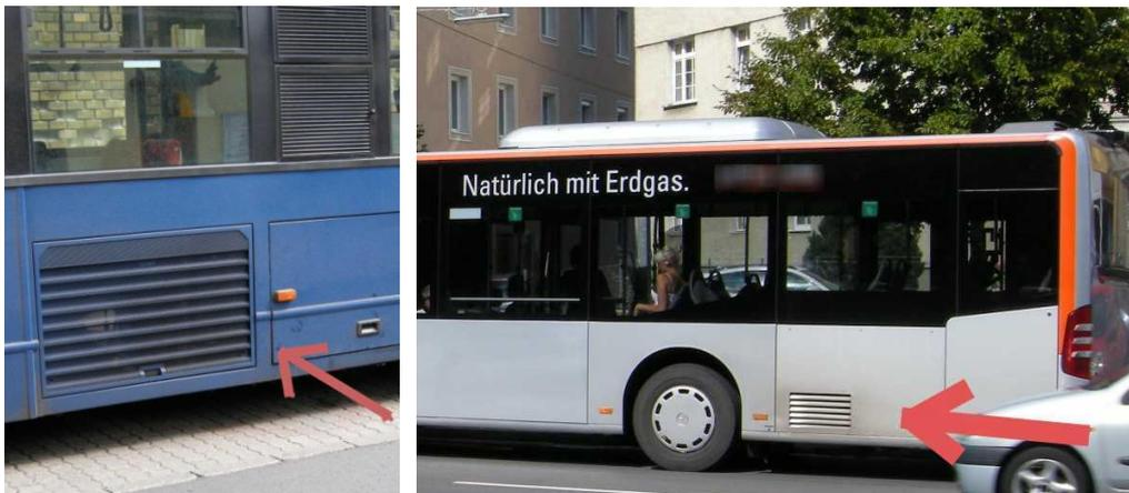
At normal operation this kind of design dramatically increase outside noise of the buses. Does not matter the bus is 40 year old or brand new construction, the engine compartment opened to the outside world and/or the engine noise not damped.
