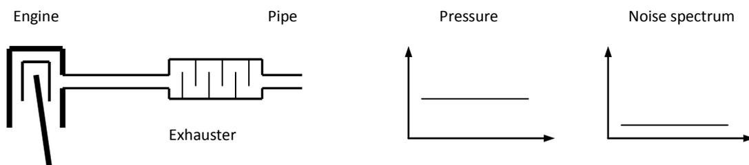
But if the exhauster modified or damaged then the efficiency of damping are less or gone. That is produce pressure and noise spectrum peaks to outside world. In that case vehicle produce more noise. That situation is showed by pictures below.
