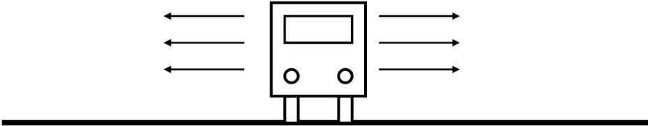
As the picture show the environment is equivalent to road on the river’s dam within the wheat field because no any acoustic reflection within 50m radius. But at road of village or city the environment are different.
