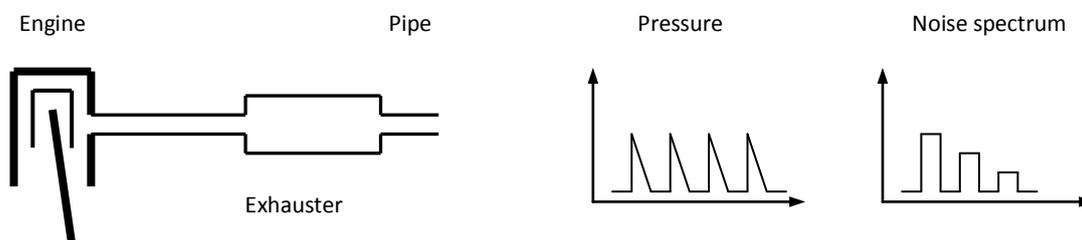
But if the exhauster removed of the exhauster pipe become broken then efficiency of damping are gone. That is produce pressure and noise spectrum peaks to outside world. In that case vehicle produce many more noise. That situation is showed by pictures below.
