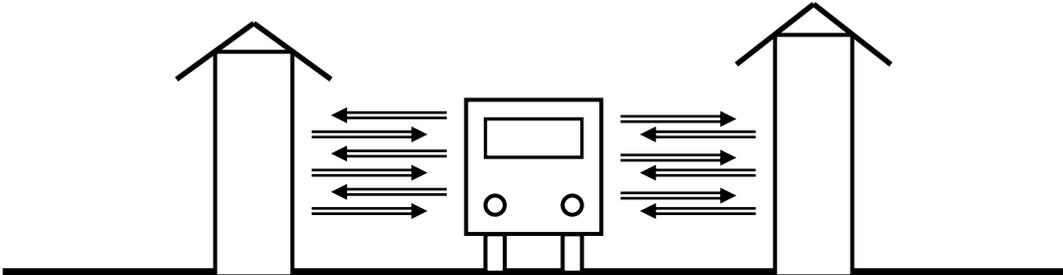
As the picture show the walls reflect and through boost the noise of vehicle. In our experience the noise of vehicle can be 15 - 20dBA higher in reflective environment than normal 92/97/EEC Figure 1 environment.
